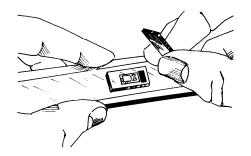
Place a silicone gum pad and backup plate (GT- 14) over the gage installation. The silicone gum should be soft (Durometer A40-60) and at least 3/32 in (2.5 mm) thick. This will allow the clamping force to be exerted evenly over the gage. The area of the silicone gum pad should be used to compute the final clamping pressure.
