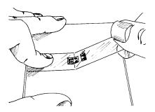
Remove the gage from its transparent envelope by grasping the edge of the gage backing with tweezers, and place bonding side down on a chemically clean glass plate or empty gage box. If a solder terminal is to be incorporated, position it on the plate adjacent to the gage as shown. A space of approximately 1/16 in (1.6 mm)
